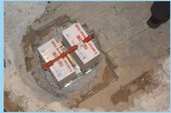
Depends on the bottom area of metallurgy's container, the area of blow-down device has to be bigger. We have found that the area of blow-down device has to equal 0.1-0.5 of bottom's area. For providing such area, the blow-down device consists of sections. Such device is called "the ShPR block".
